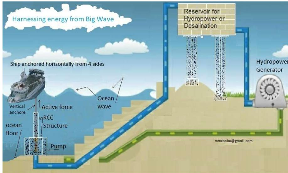
Figure 7: The vertical force of Tidal waves are pumping water to the reservoir.
