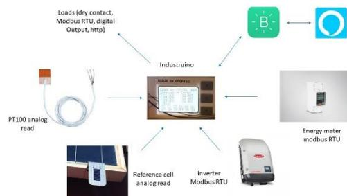
**Figure 1. SIGUE components and communication flows**
