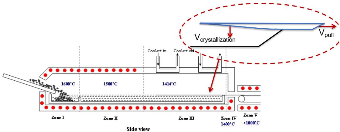
Figure 1: The Horizontal Ribbon Growth Process.
